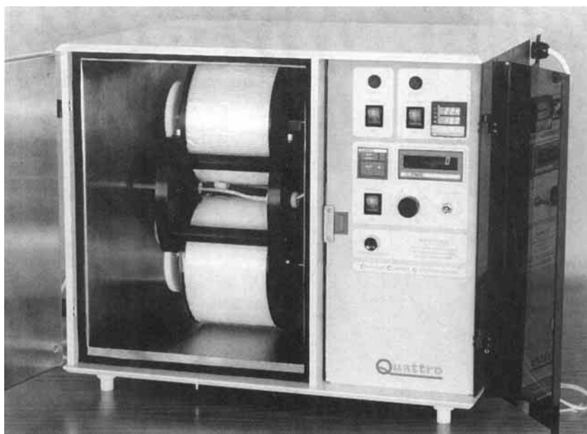
Figure 3. The Quattro CCC instrument with the rotor compartment and control panel doors open showing the twin rotor and controls.
